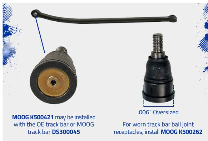
A likely cause in these situations may be looseness in the track bar ball joint. To confirm if this is the case, the track bar must be disconnected from the ball joint stud and the stud movement inspected. The stud should swing smoothly from left to right. If the stud catches, binds or quickly releases tension throughout its range of motion, the ball joint should be replaced.
